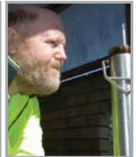
*Captain P. Bennett using custom designed draft density bucket, that prevents 'layering' error in seawater density*
