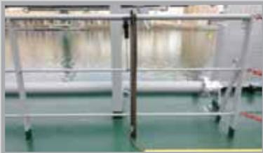
*Portable draft gauge tubes, to monitor list.*
