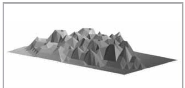
Although the technique is designed to be used out of doors, we have further enhanced this to allow us to measure undercover stockpile area. In this method we cannot use GPS as the accuracy does tend to be reduced, but we have further developed the software to allow measurements to be made by triangulation. This makes the product unique, as we are able to use the same mapping techniques, irrespective of measurement method.
